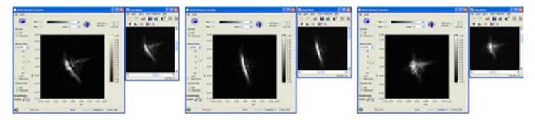
In the 3 screen captures above, taken from actual wavefront measurements performed using HASOv3, you can clearly see that the calculated PSF (larger, left-hand screen capture) is identical to the directly measured PSF (smaller, right-hand screen capture).
