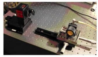
X-tilt measurement error: 1.9  $\mu$ rad rms; Y-tilt error: 2.5  $\mu$ rad rms; Linearity error: 0.09%; Wavefront quality: better than  $\lambda$ /100 rms
