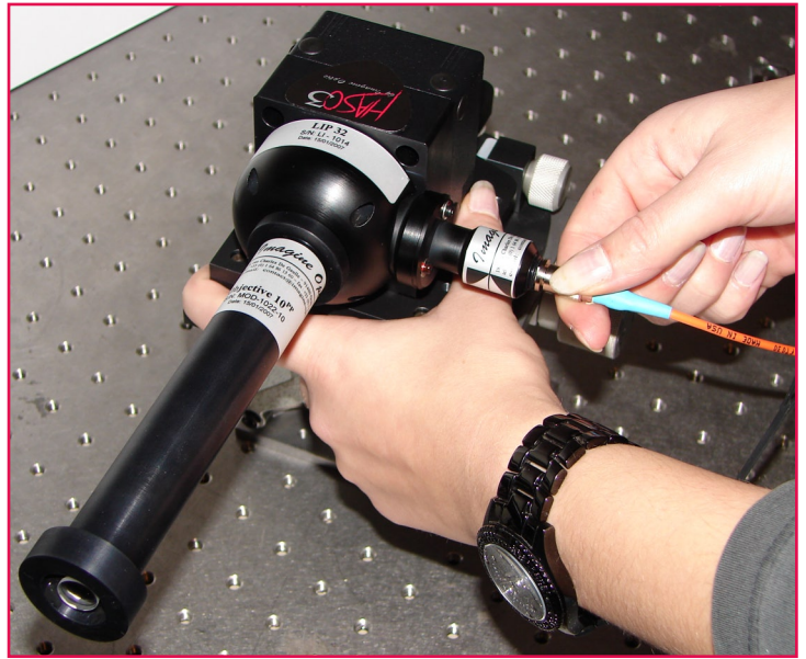
Laser Diode (included with all LIP models) being attached to a LIP 32 with an f/10 objective fitted onto a HASO 32 wavefront sensor.
