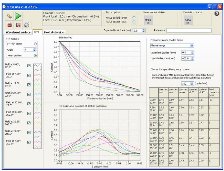
The last tab in the screen capture on the following page, labeled "Field distortion," displays a series of graphs that indicate:
